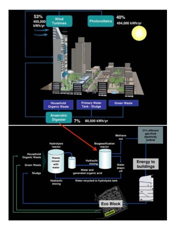
Fig. 2.50 Integrated energy generation system adopted in the project
