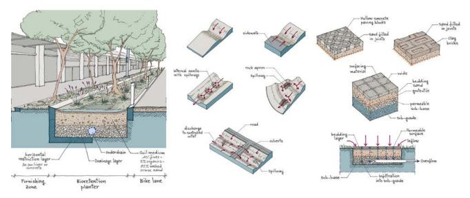
Fig. 2.29 Microbasins, swales and porous pavements
