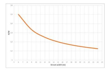
Fig. 2.14 Canyon H/W ratio to achieve full sun exposure on 21 December between 10:00 hrs and 14:00 hrs from 1st floor upwards as a function of street width, at the latitude of Yangtze river delta (30-31° N latitude
