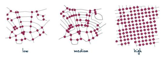
Fig. 2.5 From left to right: increasing connectivity index. A well-connected road or path network has many short links, numerous intersections, and minimal dead-ends. As connectivity increases, travel distances decrease and route options
