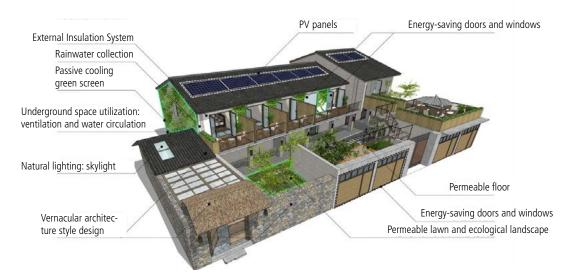
Fig. 3.10 Energy efficient technologies used in the adaptive reuse of 'Liangsu'
