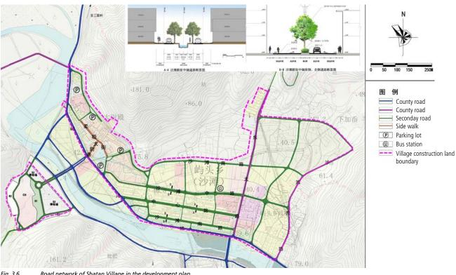
Fig. 3.6 Road network of Shatan Village in the development plan
