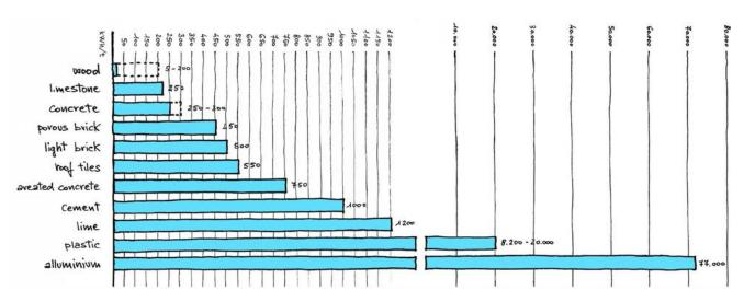
Fig. 2.17 Embodied energy for selected building materials<sup>7</sup>
