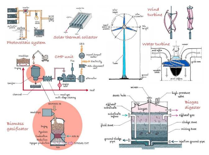
Fig. 2.22 Renewable energy technology suitable to supply a zero carbon village: Solar PV, solar thermal, mini and micro wind turbines, mini hydro plants, biomass gasification unit combined with an internal combustion engine driving an alternator for providing electricity and heat, biomass digesters for biogas production from sewage water and food waste, to be used also in a CHP system.
