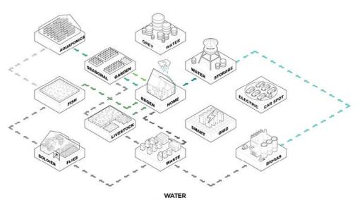
THE WATER PRODUCTION FROM THE BIOGAS FACILITY IS ADDED TO THE WATER STORAGE.
