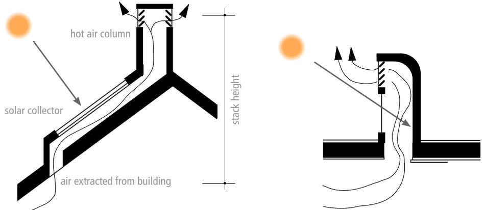
The heated air rises and escapes to the outside. This causes internal air to be pulled into the heated space and expelled thus enhancing airflow.
