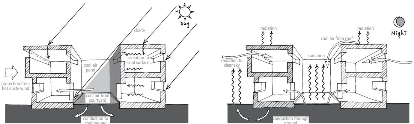
Courtyards are excellent thermal regulators. High walls cut off the sun, except for around midday, and large areas of the inner surfaces and floor are shaded during the day. During the night the heat accumulated during the day is dissipated by re-radiation.
