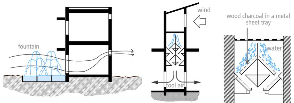
Fountains, sprays, pools and ponds are particularly effective passive cooling techniques. Hot air is channelled over the water before it enters the building.
