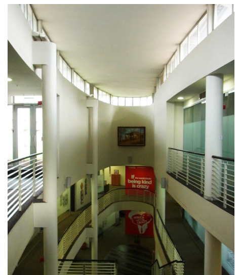
Natural lighting and natural ventilation through stack effect © UN-Habitat / Zeltia Gonzalez Blanco
