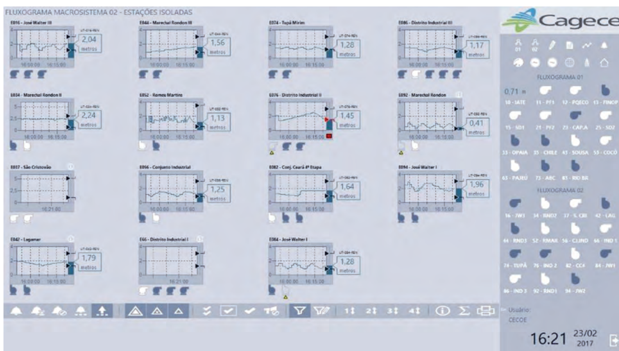
Figure 2.8 Highly Severity Warning-Low Sewage Level at Station 076
