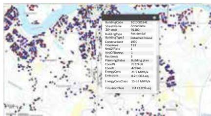
Fig. 1 Zoomed view of the provided building-specific information in LIITERI. Colored points represent buildings, and the color indicates the building type: e.g. blue for residential buildings, yellow for office buildings, red for other types of buildings.
