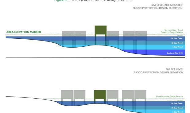
Figure 8: Proposed Sea-Level Rise Design Elevation
