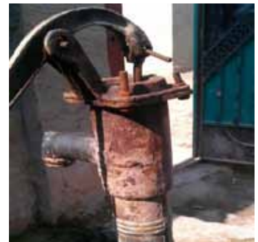
Figure 39: Hand pump in Sindh destroyed by groundwater salt
