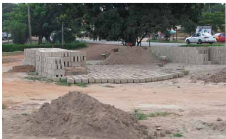
Figure 59. Manufacturing sandcrete blocks Photo © G Tipple
