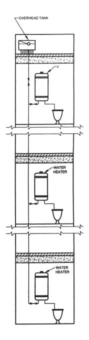
FIG. 12 NON – PRESSURE TYPE INSTALLATION
