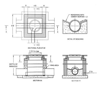
FIG. 14 DETAIL OF MANHOLE (DEPTH LESS THAN 3 FEET)
