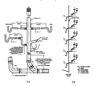
FIG. 2 SINGLE STACK SYSTEM – MAIN FEATURE OF DESIGN
