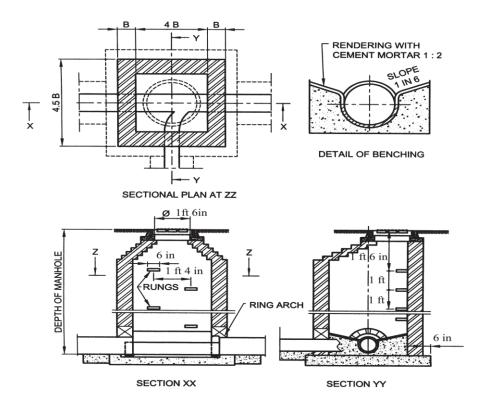
FIG. 15 DETAIL OF MANHOLE ( DEPTH 3 FEET AND UP TO 8 FEET )
