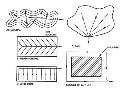
FIG. 19 DETAILS OF DRAINAGE SYSTEM
