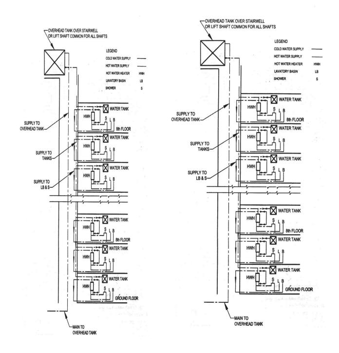
FIG. 11 INSTALLATION FOR 8 – STOREYED BUILDING WITH INDIVIDUAL WATER TANKS
