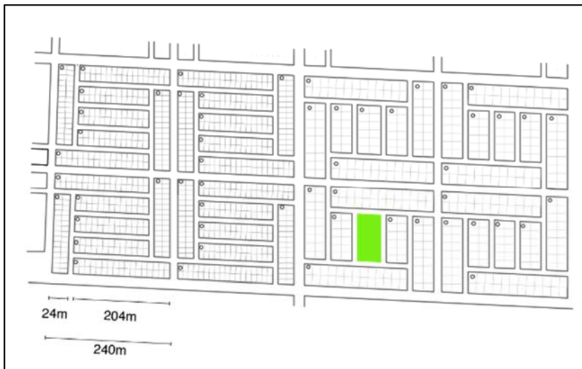
FIGURE 1: PLOTTING AND GRID PATTERNS IN SETTLEMENT EXTENSION AREAS IN KALAY
