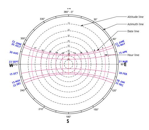
Solar control through shading devices is most effective when designed specifically for each façade, since time and duration of solar radiation vary with the sun's position in the sky - its altitude and azimuth.
