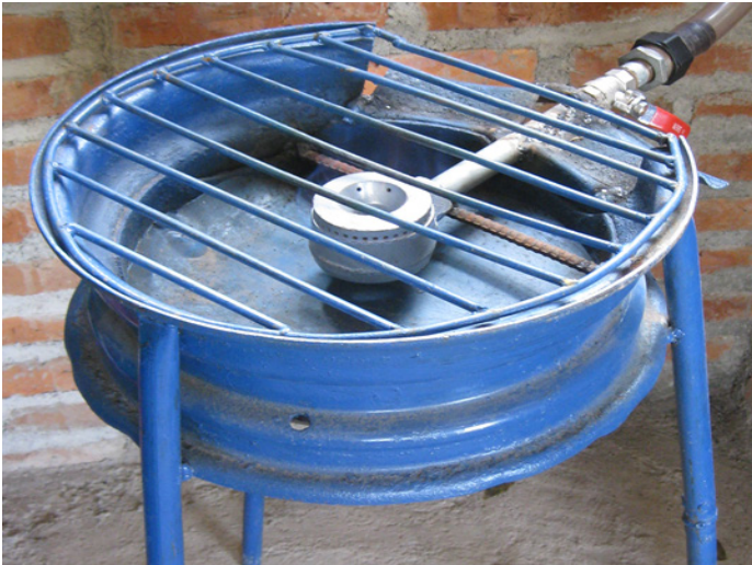
Fig. 04: The gas generated is applied in cooking and the sludge is a soil additive
