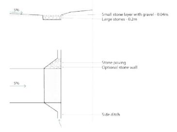
fig.177. Secondary drainage - crossings
