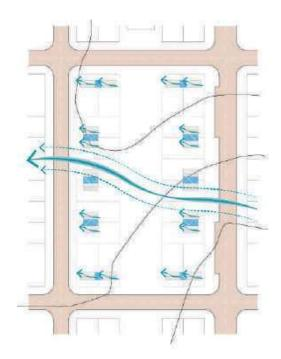
fig.154. Prevailing wind advantage for cooling
