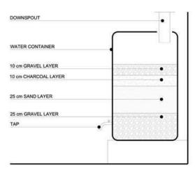
fig.164. Example of homemade water filtration system
