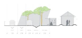
fig.75. Typical street section emphasizing shaded spaces
