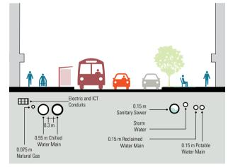
Diagram showing utilities installed adjacent to roadbed.
