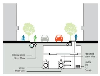
Diagram showing utilities installed in an underground corridor.
