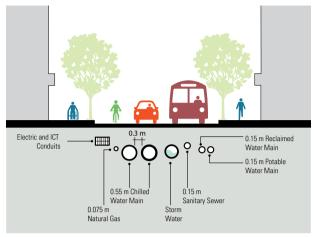
Diagram showing utilities installed under the roadbed.
