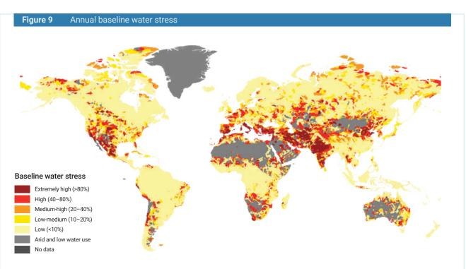
Note: Baseline water stress measures the ratio of total water withdrawals to available renewable water supplies. Water withdrawals include domestic, industrial, irrigation and livestock consumptive and non-consumptive uses. Available renewable water supplies include surface and groundwater supplies and considers the impact of upstream consumptive water users and large dams on downstream water availability. Higher values indicate more competition among users.
