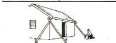
Hurricane preparedness: shuttering windows, building protective screens in front of openings and bracing corners of buildings
