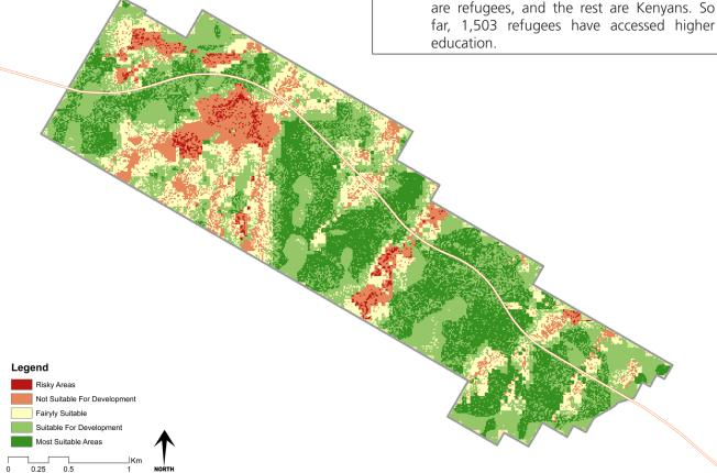
Figure 210 Weighted Analysis of Suitability in planning site<sup>1</sup>
