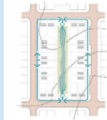
fig.150. Sustainable drainage design
