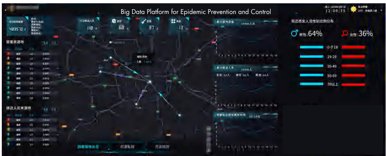
Figure 2: Urban Epidemic Prevention and Control Big Data Platform Developed and built based on high-definition mapping, GIS and data processing technologies, focusing on the entry and exit of people in transportation hubs and the quarantine situations of the people arriving in the city. Five dashboards Pandemic Overview, Transportation Hub, Highway, City Control, and Transferred People Tracking through visualization tools and visible on the platform.
