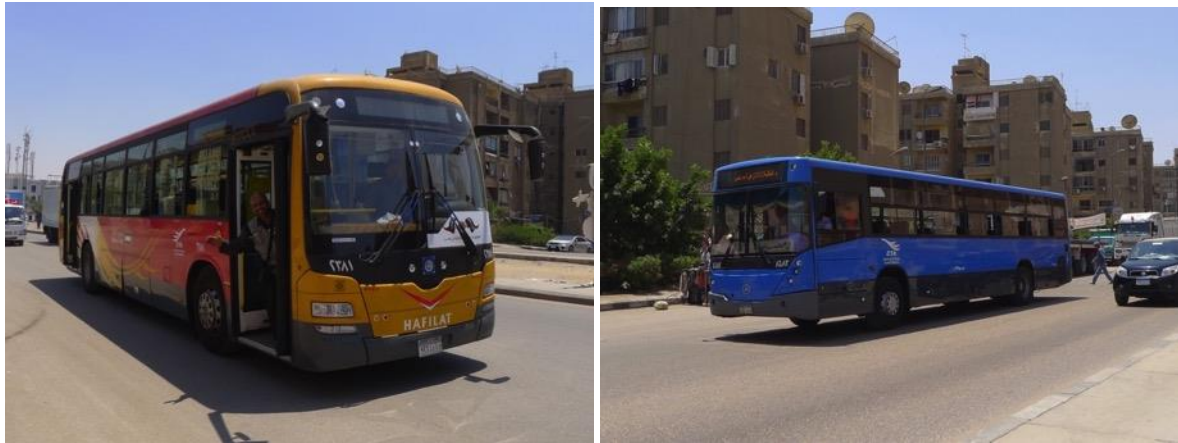
Figure 3: The Cairo Transport Authority (CTA) operates buses across routes in Cairo, Giza, and the new communities. The entire fleet consists of high floor buses with stepped entry.
