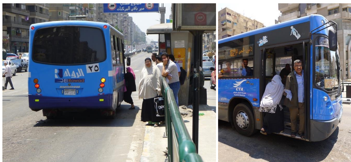
Figure 22: Steps inside buses and minibuses present a challenge during boarding and alighting, especially for elderly passengers, persons with disabilities, and women with children.
