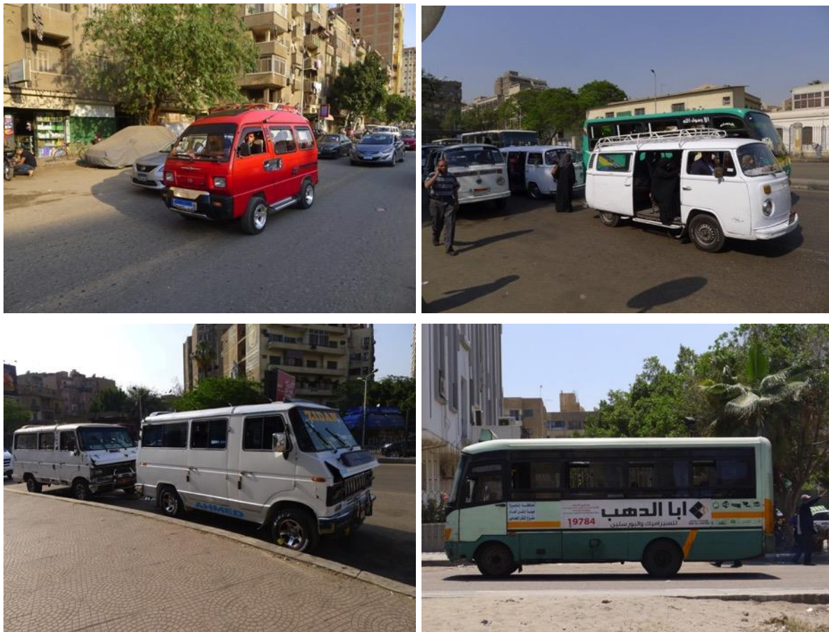
Figure 4: Paratransit vehicles in Greater Cairo range from 7-seat vans to 29-seat minibuses.
