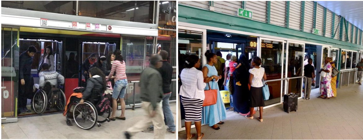
Figure 34: BRT stations should incorporate level boarding to ensure seamless access between stations and vehicles.
