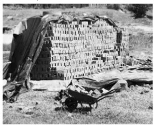
FIGURE 79 A clamp of about 12,000 bricks during their burning, Maseru East
