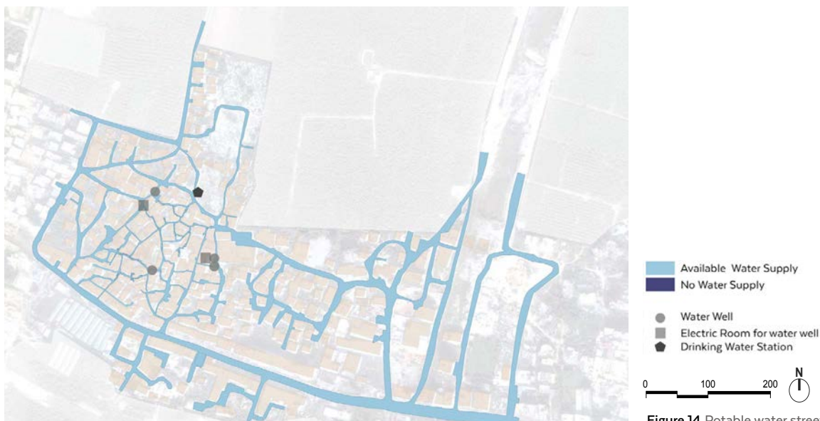
Figure 14 Potable water street mapping
