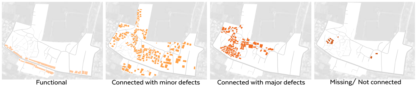
Figure 19 Buildings connection to electric network
