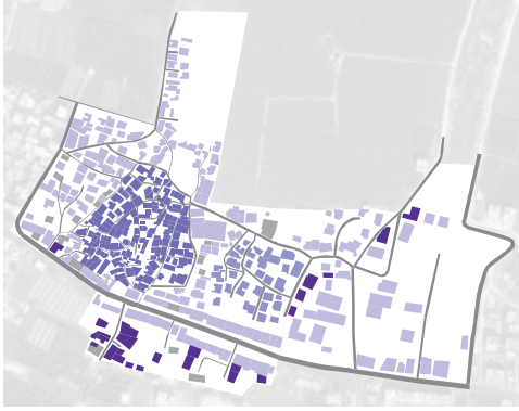
Figure 39 Building connections to wastewater network (phased response)
