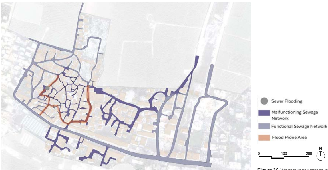
Figure 16 Wastewater street mapping
