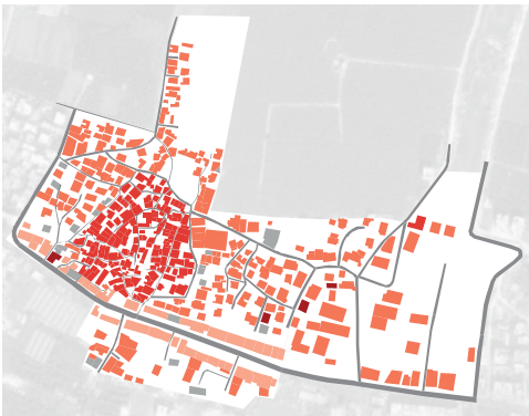
Figure 40 Building connections to stormwater network (phased response)
