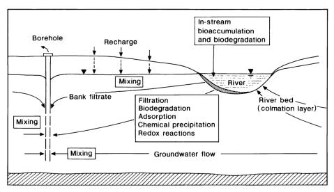
Figure 1: Basic scheme of riverbank filtration and main attenuation processes [1]
