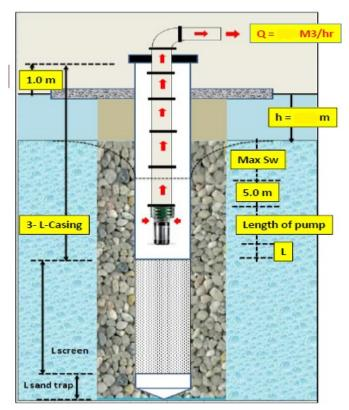
Figure 56: Typical RBF well components
