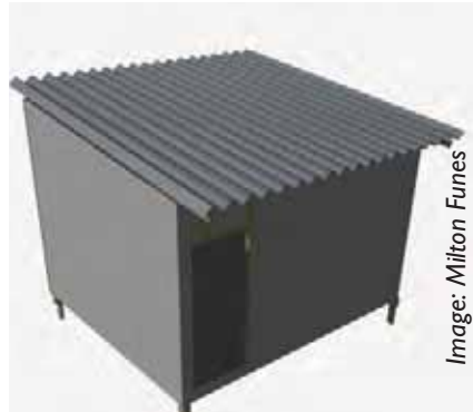
Computer model of the shelter with a corrugated iron roof and plastic sheeting walls
