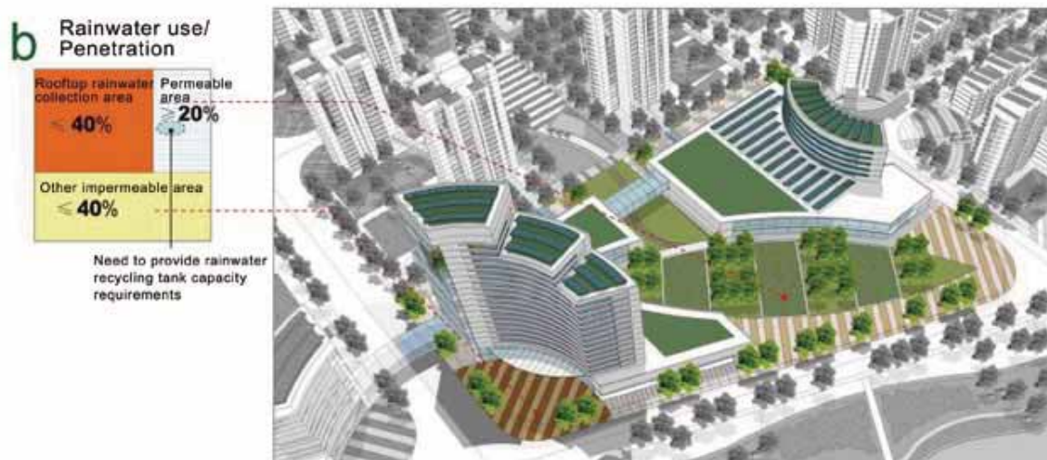
Map 6-21 Water Resource Control Indicators of the Control Plan
