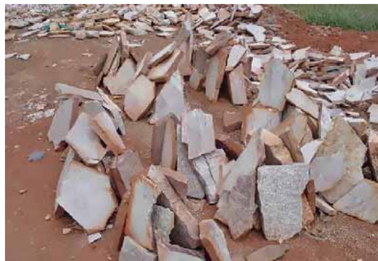
Figure 31. Stone used in the construction of drainage channels and house cladding.
