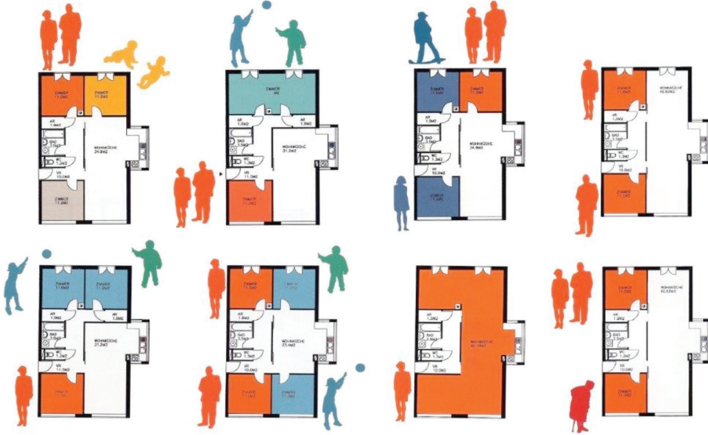
Layouts of the different flats of Frauen-Werk-Stadt I. Source: City of Vienna
